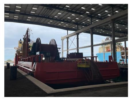
Reel Drive System (RDS) at B-Port base in Açu Port
