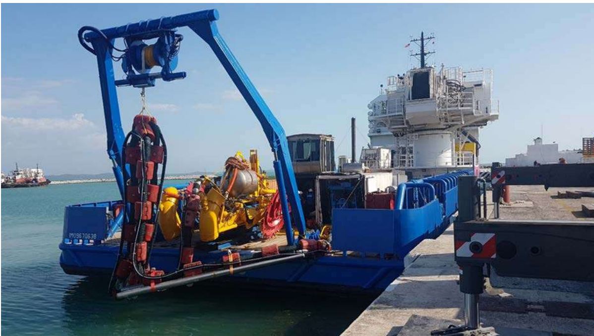
TSV equipped with trenching spread
