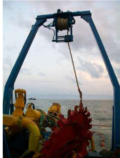
Rossana Trimaran shallow water barge equipped with A-frame
