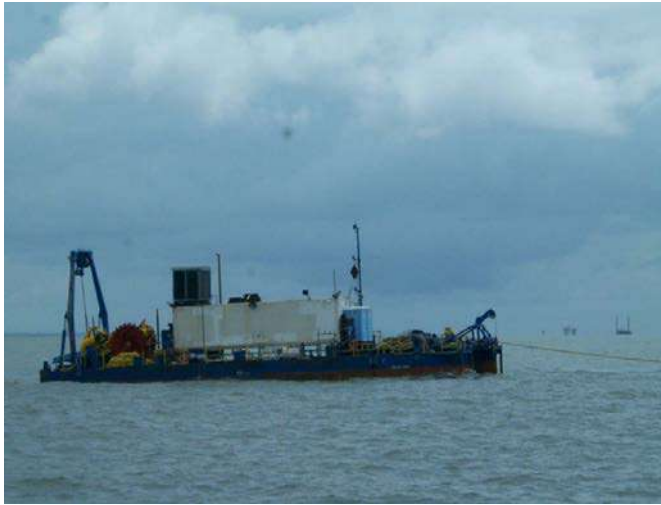
Rossana Trimaran shallow water barge equipped with A-frame
